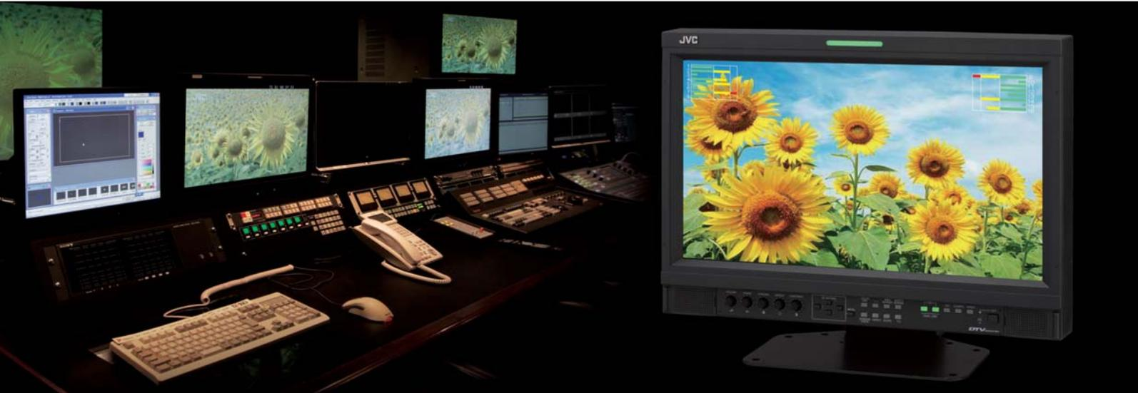
Near EBU Grade 1 LCD monitor, offering outstanding colour gamut, gamma and greyscale characteristics. The DT-V17G15 enables accurate viewing of colours and image quality of HD broadcast footage, providing confidence in the knowledge that what's displayed in the studio is what consumers will see at home.
